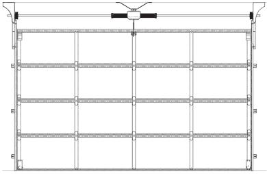
Max door height: 3.5m, Max door weight: 110kg, Max door area: 12m<sup>2</sup>
